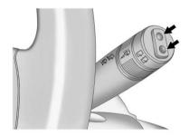
Press the upper or lower portion of the button to control the rear wiper and rear wiper delay. The system turns off when the button is returned to the middle position.
